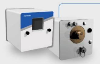
The DGA 1009 is a permanently installed multi-gas-in-oil analysis system with transformer monitoring functions. It individually measures, Moisture in Oil (H2O) and the key gases Hydrogen (H2), Carbon Monoxide (CO), Carbon Dioxide (CO2), Methane (CH4), Acetylene (C2H2), Ethylene (C2H4), Ethane (C2H6) and Oxygen (O2) dissolved in transformer oil.
