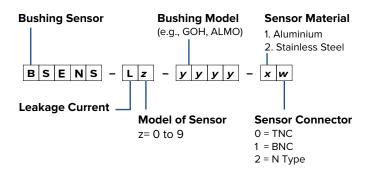
BUSHING SENSOR- PARTIAL DISCHARGE
