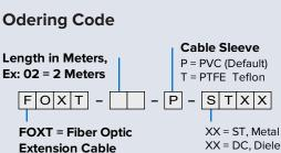
XX = ST, Metal Connector (Default) XX = DC, Dielectric Connector at one end
